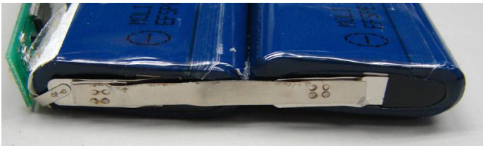
Half moon shape of the welds indicate that the weld process for used for this battery is not optimal
