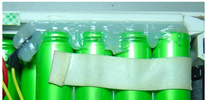
Excess silicone insulation can block safety vents
