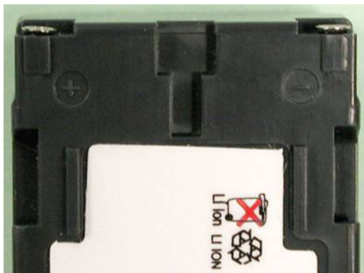
Terminals standing out from the enclosure
